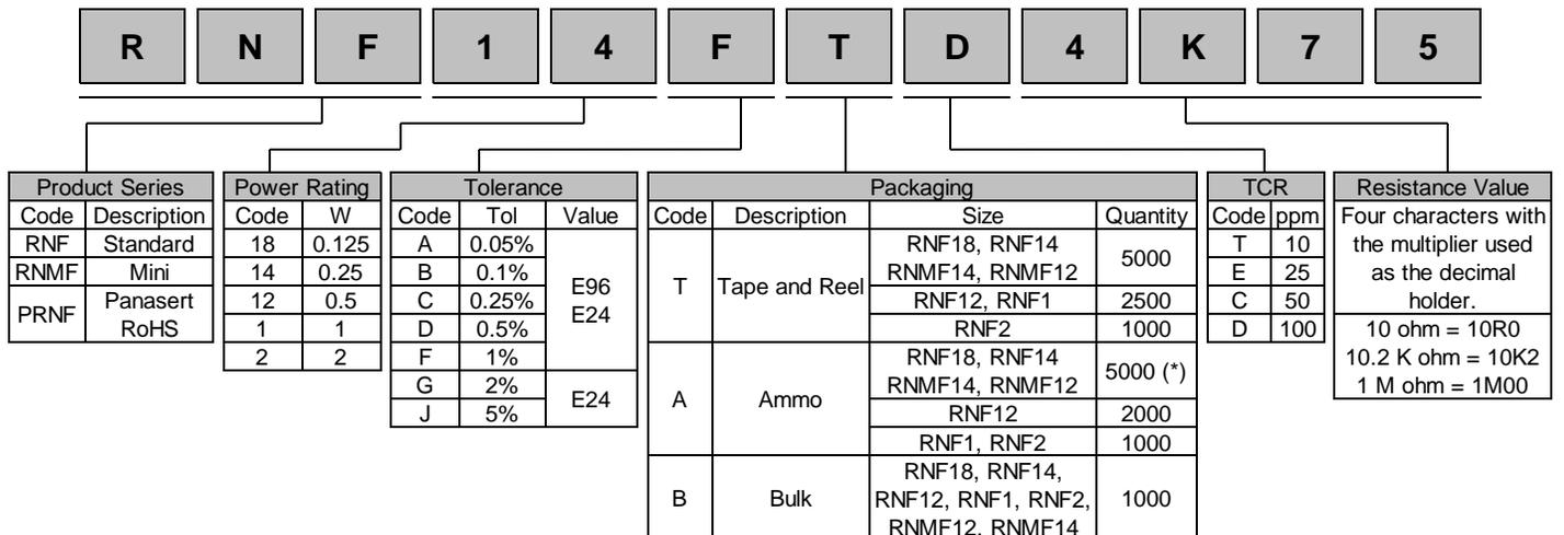
(\*) Precision metal film resistors with tolerances <1% may be available in smaller quantities. Contact Stackpole for more details.
