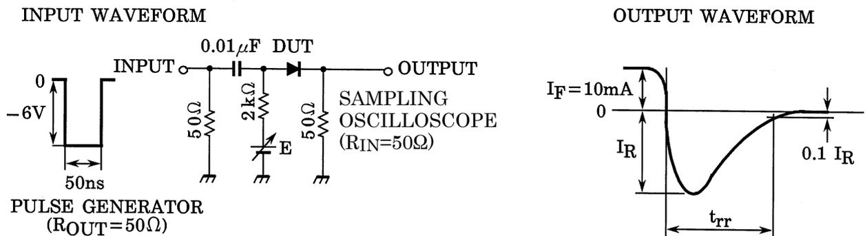
Fig.1 Reverse Recovery Time (t<sub>rr</sub>) Test Circuit
