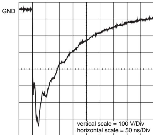
unclamped -1 kV ESD voltage waveform (IEC 1000-4-2 network)
